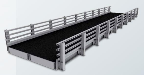
Each Beam Bridge unit has a width of 1.5 or 2.1m. By joining the units side to side, any required road width within the modules can be achieved (3.0m - 3.6m - 4.2m - 4.5m - etc). The outer units can be equipped with parapet rails and kerbs or pedestrian fencing. The units are available in depths of 300mm and 450mm and have an integrated anti-skid surface consisting of epoxy resin embedded with aggregate.
