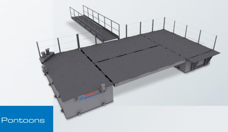
The Janson Couple Pontoons are designed to be transported in standard trucks. They are lowered into the water by crane, using the upper couplers as lifting lugs. Once on the water, because of the simplicity and effectively engineered coupling systems, the pontoons can be quickly coupled without any mechanical assistance from deck level with 2 unskilled operatives positioned on each pontoon.
