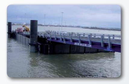
Janson's RoRo systems embody the synergy advantages by combining Janson's modular pontoons, creating a floating platform and a link span from Janson's modular bridge units. It is the ideal solution in seaports with tidal movements, to facilitate the loading and discharging of marine vessels.
