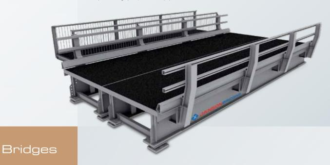
Each unit has a width of 2.5 or 3.5m. By joining the units sideways any required road width within the modules can be achieved (3.5 - 5.0 - 6.0 - 7.0 - etc.). The exterior units can be equipped with parapet rails and kerbs or pedestrian fencing. The units are built from steel trusses with integrated steel trough decks which have an integrated antiskid surface consisting of epoxy resin embedded with aggregate.
